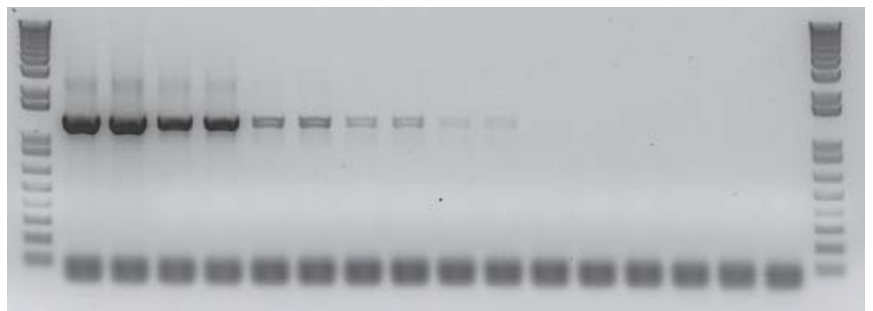
Template-sensitivity of PCR with ROVALAB Taq polymerase and dNTPs Template: Human Genomic DNA (ng/ \mu l) ER (1,233 bp)
